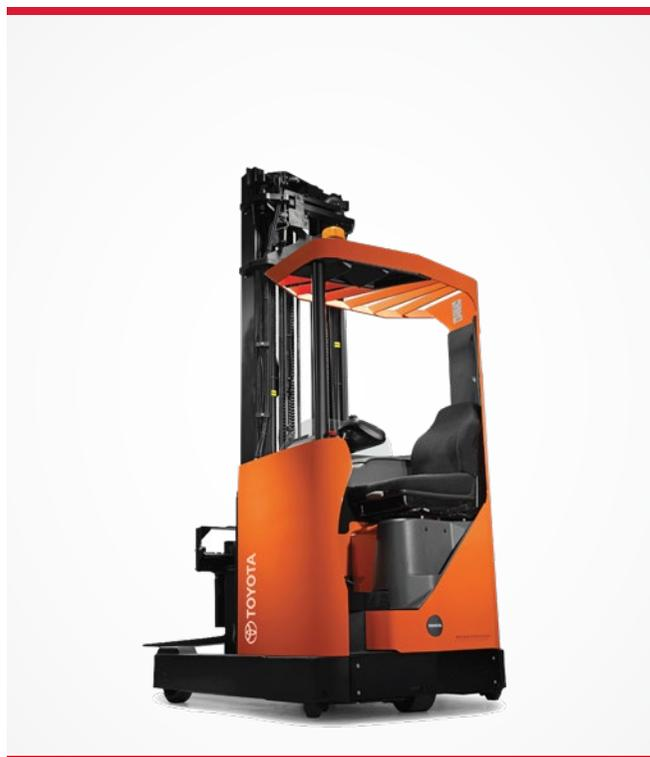
Designed to fit in confined areas, for block stacking and specialised racking
