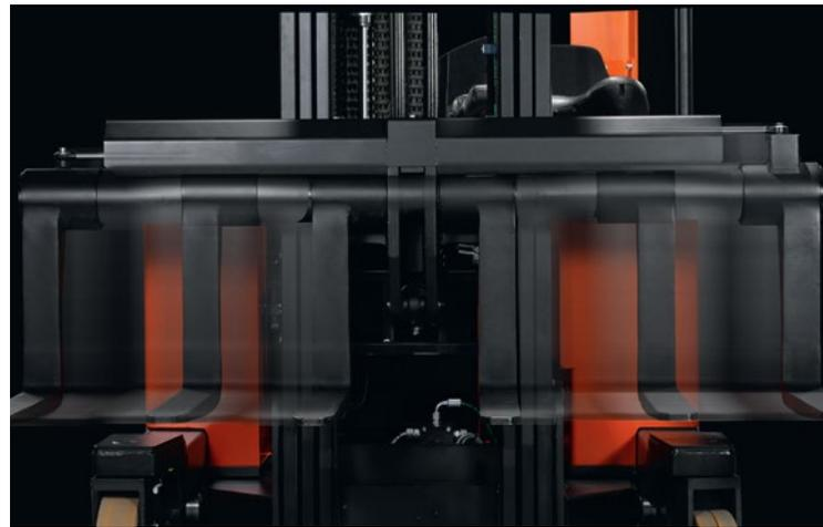
Reflex F-series' hydraulic fork spreader quickly adapts the truck to loads of different dimensions
