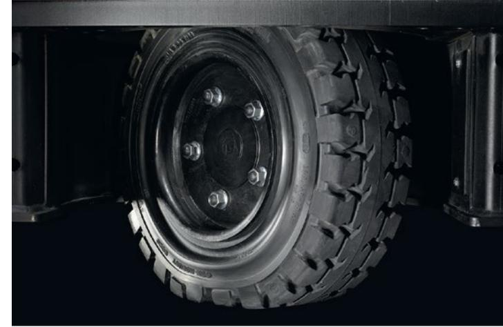
Superelastic tyres on all wheels and 145 mm ground clearance mean the Reflex O-series can handle outdoor surfaces, including gradients and transitions.
