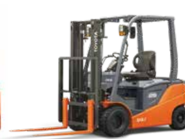
8-Series 4-wheel Battery-Electric Models#
