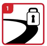
On Toyota 4-wheel forklifts if the forklift becomes unstable during turn, the rear axle will lock automatically. This helps to prevent side tip-over by adjusting the orklift's centre of gravity.
