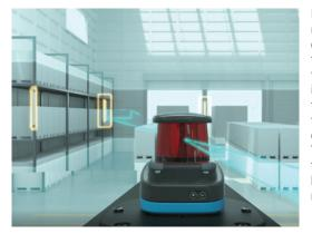
Reflector navigation is a navigation method in which consistent and high-contrast targets, reflectors, are added to the environment. The reflectors installed in the warehouse allow the scanner on the automated truck to define its position based on its distance to the reflectors. The characteristics of this technique guarantee robustness, high accuracy and long reach in most environments.
