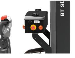
E-stop buttons easily reachable for operators in workplace
