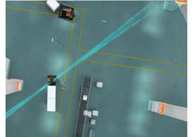
Natural navigation is an alternative navigation technique for warehouses where the surroundings remain fairly constant. The truck can utilise the existing environment to navigate without reflectors, avoiding extra cost and additional equipment. A unique benefit from Toyota is the fact that the Autopilot can switch seamlessly between natural and reflector navigation depending on the area it's in we call this dual navigation.
