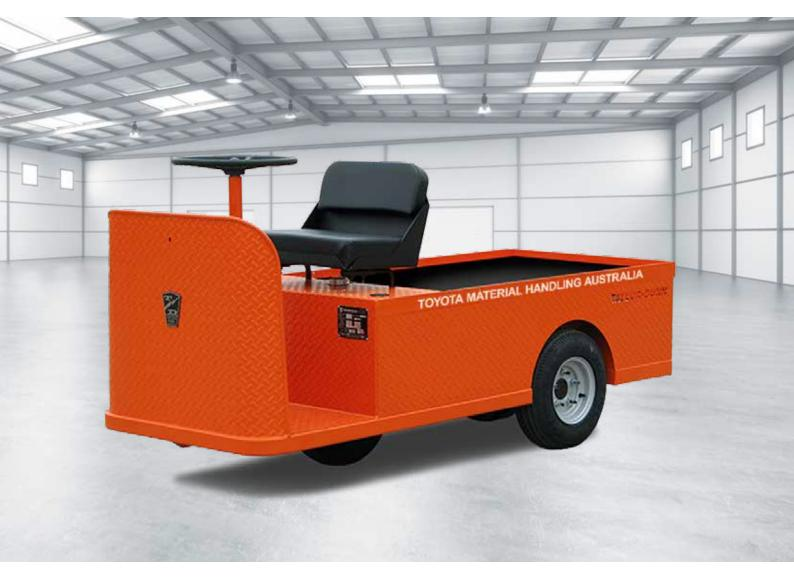
Our three-wheel design allows the C-432 to provide the shortest turning radius available in a sit-down combination burden carrier / tow tractor. With its 71 cm wheelbase, this vehicle can maneuver into corners other powered vehicles simply cannot reach.
