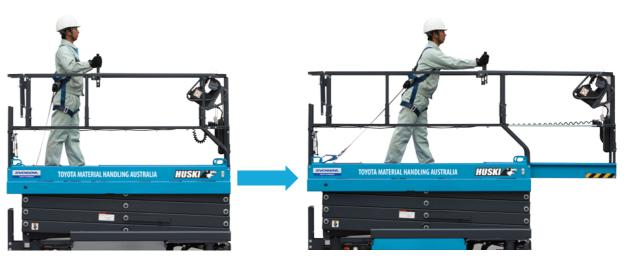
The platform deck can be extended for greater reach to get closer work areas, even if objects on the road are blocking the chassis from the site area.
