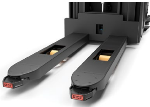
Mechanical fork bumpers for safety in narrow aisles
