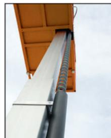
The mast made of a special extruded aluminium is 100% maintenance free! No more chains to be regularly inspected, no more grease or lubricant required, no maintenance: a real low cost ownership!
