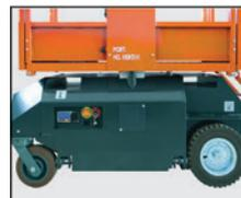
All-steel chassis design, with heavy-duty winch, tie down and lifting points-making life easier for Transportation! Built in tilt-sensor & active pothole protection for an increased ground clearance.
