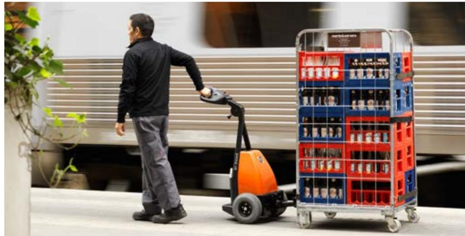
These pedestrian-operated units can be used as part of an integrated handling process, to take care of heavy load movement.
