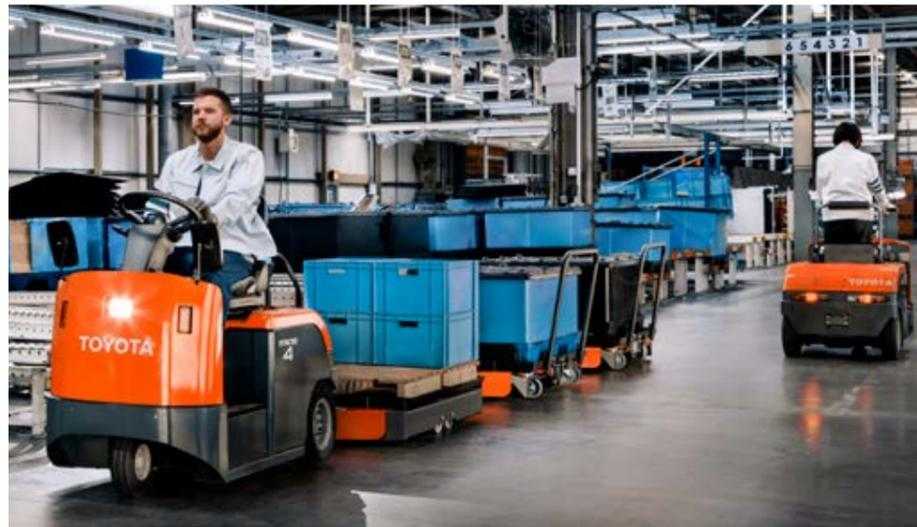
Pneumatic tyres mean smooth driving on uneven surfaces, to aid operator comfort. The compact design of Toyota Tracto S-series models allows them to work efficiently in confined spaces, and the narrow chassis width is ideally suited to driving in narrow traffic lanes where multiple load movements are taking place.
