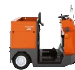
Heavy-duty CBTY models offer capacities of 4 and 6 tonnes and are particularly suited to applications with gradients
