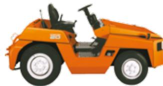
Heavy-duty 2TG/D models are equipped with either diesel or LPG engines, and offer towing capacities up to 49 tonnes, with travel speeds up to 30 km/h
