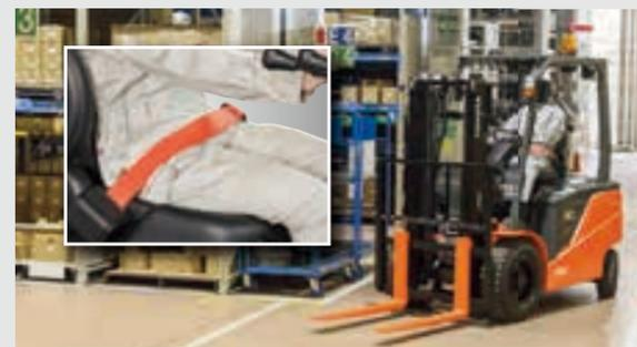
Easy to determine whether your operator's seat belt is properly fastened.
