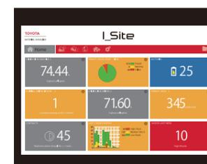
Visualizes a wide range of data such as vehicle operations by each operator, detected shocks and battery usage.
