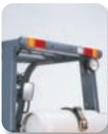
Optional high mount rear combination lights are integrated into the overhead guard, making stops and turns highly visible in the workplace.
