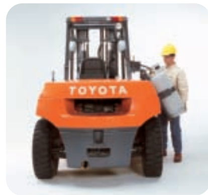
Swing-out or optional swing-down LP tank bracket enables the changing of LP tanks to be quick and easy, without forcing the operator to reach over the counterweight and risk back strain.
